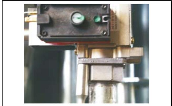
i) Secure the mixer with its mounting plate and inlet pipe to the fan.
