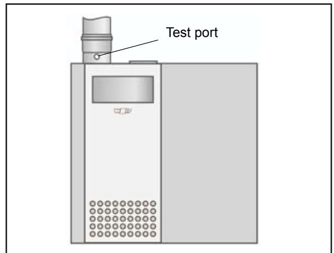
Fig.: Flue gas test at the integral test port.
