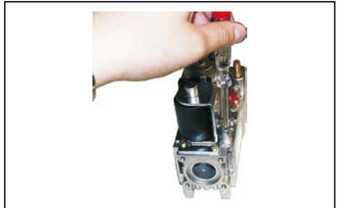
Fit the gas pressure limiter to the new gas combination valve.
